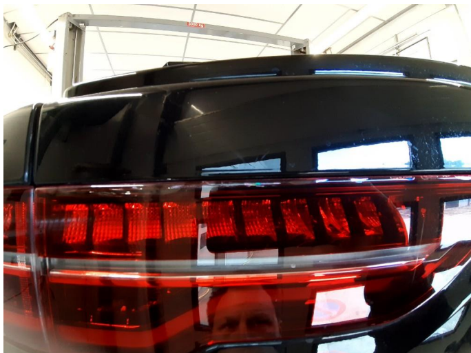
1.1 Defekt / sprukket glass
