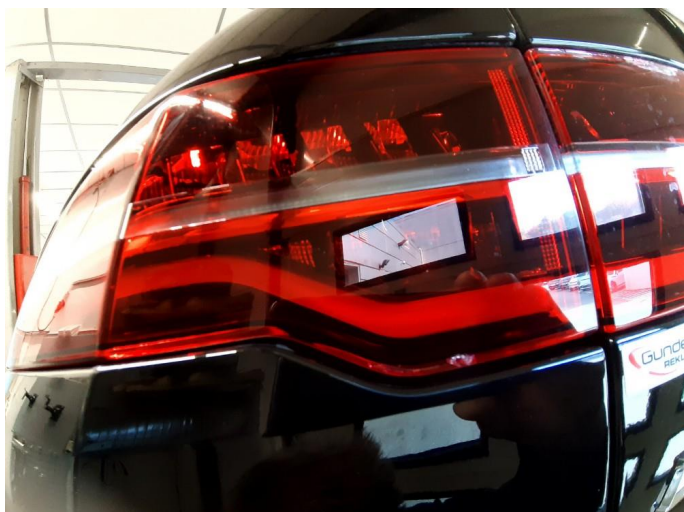
1.1 Defekt / sprukket glass
